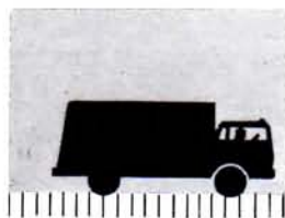
H-10 LOADING For fork lifts, truck cranes with pneumatic tires and light trucks. Use the H-10 loading chart.
