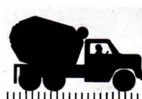
H-20 LOADING Heavy trucks such as concrete mixers, warehouse trucks and tractor trailers. Use the H-20 loading chart.
