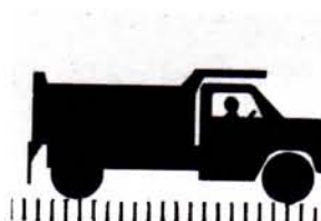
H-15 LOADING Industrial truck cranes with pneumatic tires, heavy fork lifts, dump trucks, and high lifts. Use the H-15 loading chart.
