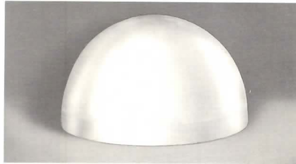
Above: Hemispherical Flanged Head, 66" I.D., 3/8" Thick, 33" Spherical Radius, and 4" Straight Flange.
