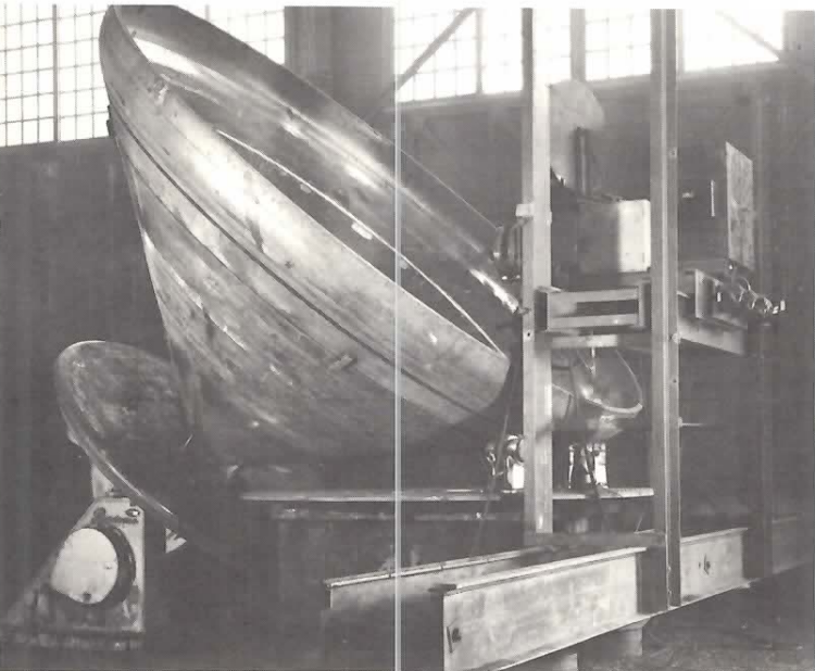
Automatic Welding Machine set up to make a weld on a Conical Head.
