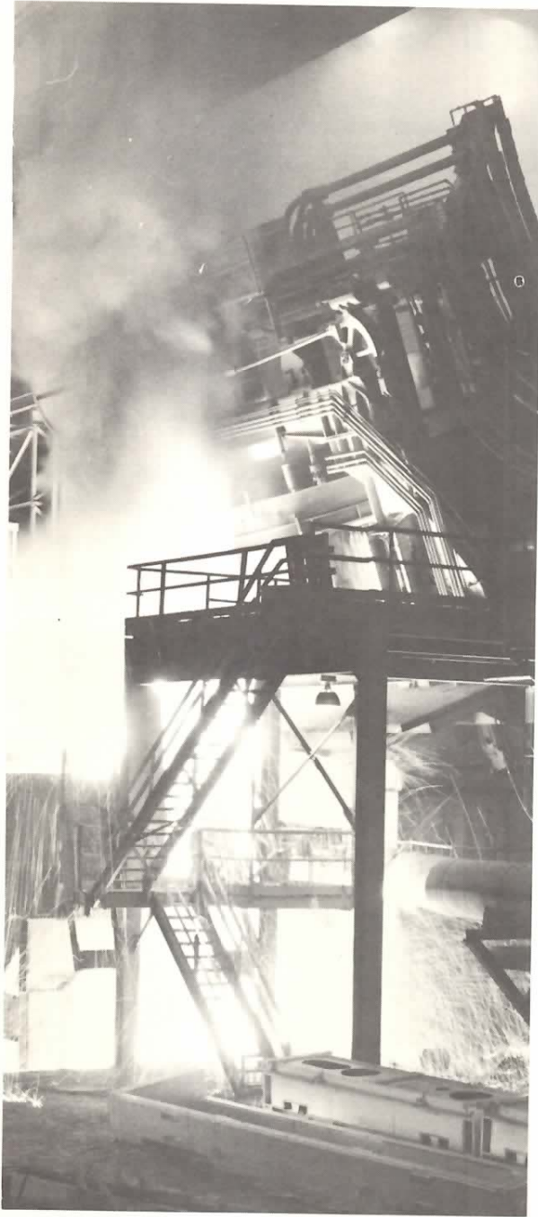
Electric furnace tilts forward during pour of 150-ton heat.
