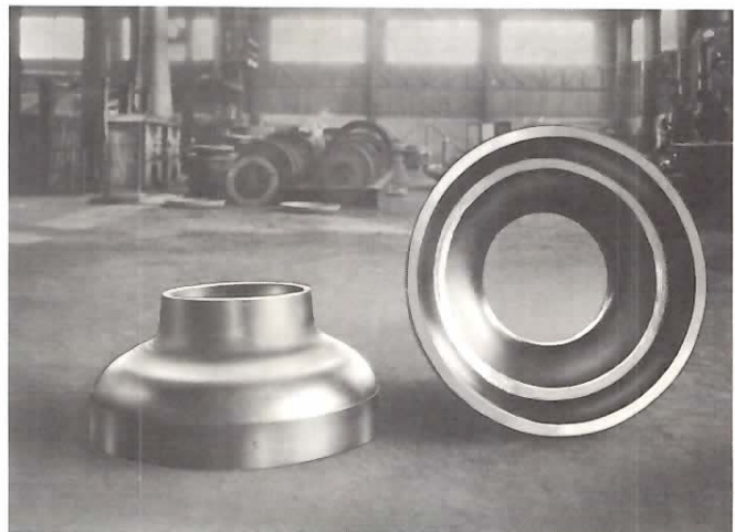
Dome Heads 55 \frac{1}{2} " O.D., 2 \frac{1}{4} " Thick and 7" Straight Flange, with flued opening in center.
