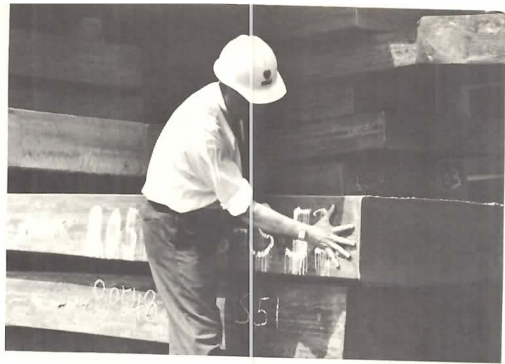
Three sizes of continuous cast slabs are produced - 6" x 60", 10" x 60" and 12" x 80", the world's largest when first cast in 1969.
