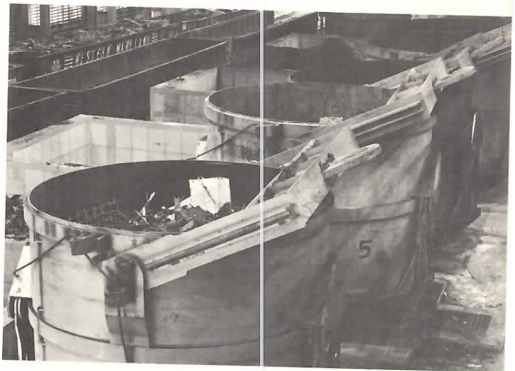
Scrap cars are unloaded into storage bins (center) or directly into charge buckets (right) in highly automated scrap aisle of electric furnace melt shop.
