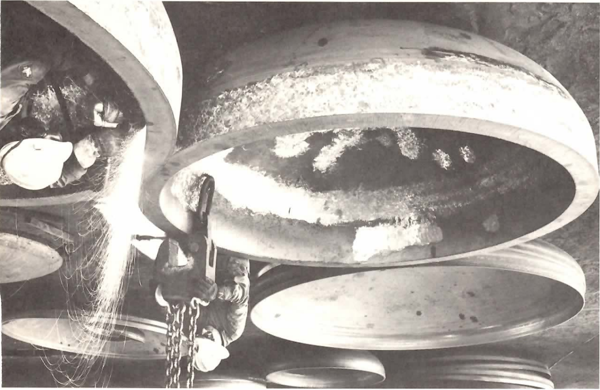
Elliptical dished heads on shop floor. Foreground bottom—211-1/2" I.D.; foreground top and background center—174" I.D.; background right—192" I.D.
