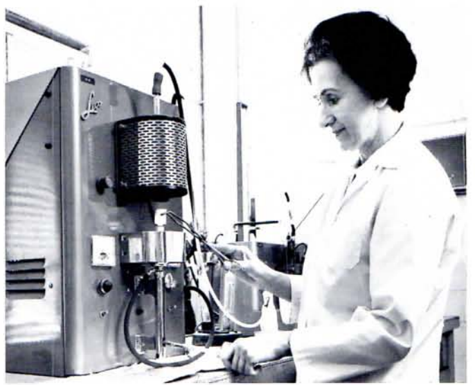
Percent of carbon in specimen of 316 stainless steel is measured with carbon gravimetric test. Sulphur content is also determined in this area of laboratory.
