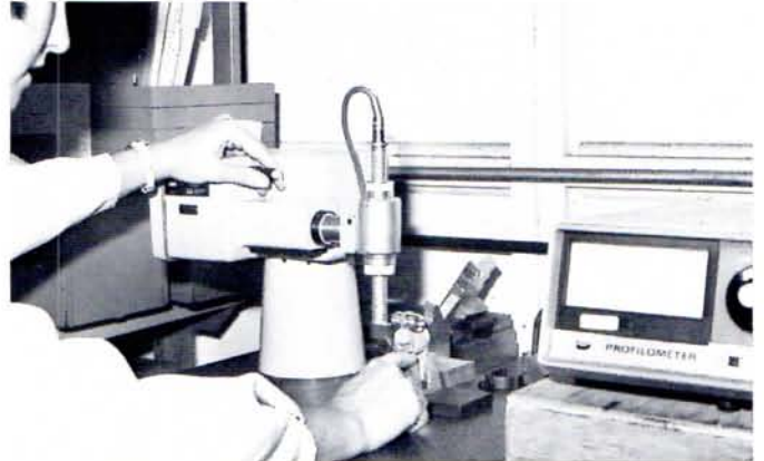
Using a profilometer, technician measures surface finishes on I.D.s of straight fitting to within 10 microns.
