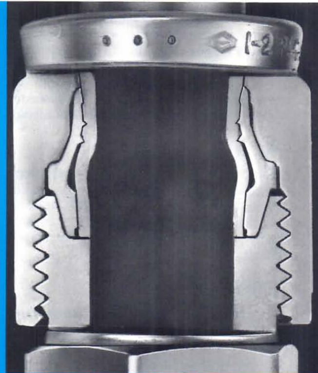
Photograph of Hi-Seal Fitting after repeated remakes. Note the second tooth now gripping tube.
