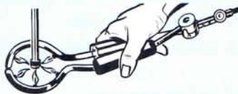
BRAZE-SEAL TORCH simplifies installation.
