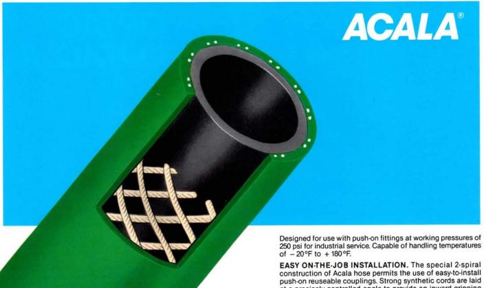
**SPECIFICATIONS** WEIGHT MAX. WP I.D. x O.D. lb./ft. mm MPa kg./m. in. psi 1/4 x .504 250 1.7 .08 .12 6.4 x 12.8 .18 .646 9.5 x 16.4 250 1.7 .12 3/8 X .772 12.7 x 19.6 250 1.7 .17 .25 1/2 X 1.7 .34 % x .937 15.9 x 23.8 250 .23 % x 1.079 19.1 x 27.4 250 1.7 .28 .42
