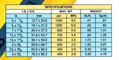
Ultrabraid Flexsteel Air is Goodyear's top quality air hose built to withstand severe service. It is designed for use where extra strength is needed to handle heavy duty requirements in mines, quarries, and industry.
