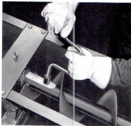
Simply disconnect the REDI-CHANGE section — clamping keys and hanger.
