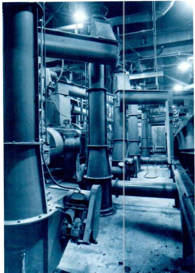
Rubber reclaiming operation uses high capacity, compact Screw-Lift and screw conveyor system to transport rubber back and forth between mills and screener.
