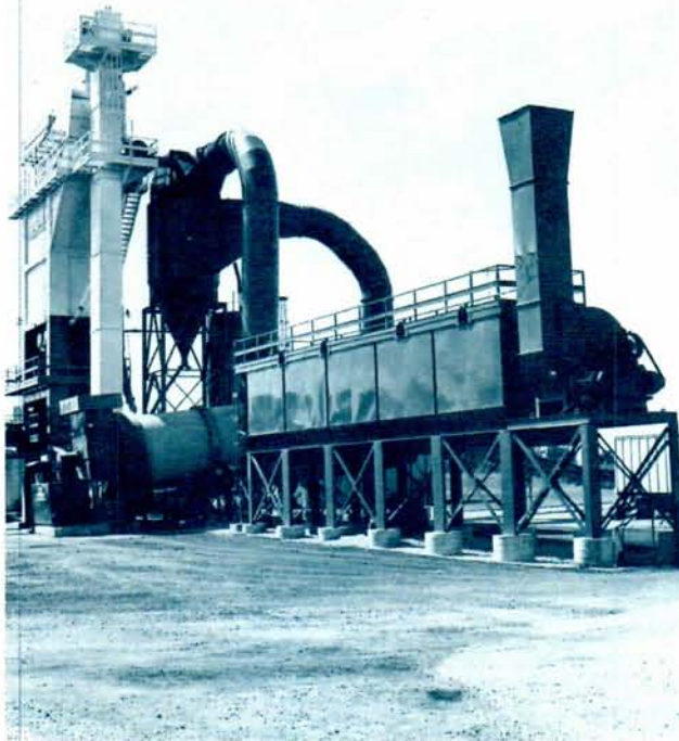
This asphalt fabric filter type dust collector uses Screw Conveyor flighting in the hoppers which return collected fines to the mix.
