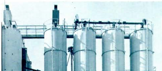
Partial view of a large outdoor installation employing Screw-Lifts to elevate material to fill storage silos.
