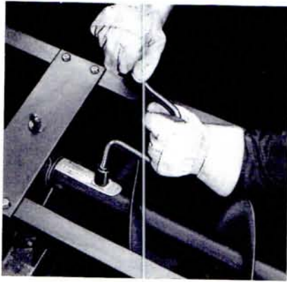
Simply disconnect the REDI-CHANGE section — clamping keys and hanger.
