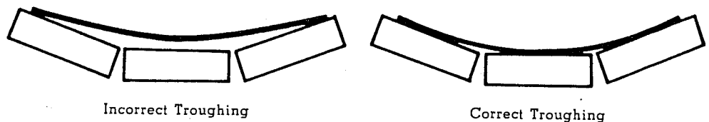
FIGURE 7.11. Incorrect and correct troughing.
