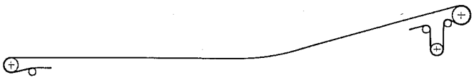
FIGURE 2.3. Horizontal and ascending path, when space will permit vertical curve and belt strength will permit one belt.
