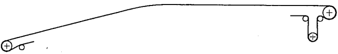
FIGURE 2.4. Ascending and horizontal path, when belt tensions will permit one belt and space will permit vertical curve.
